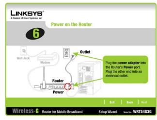
Figure 7-8: Power on the Router Screen
